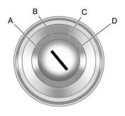
The ignition switch can be turned to four different positions.
